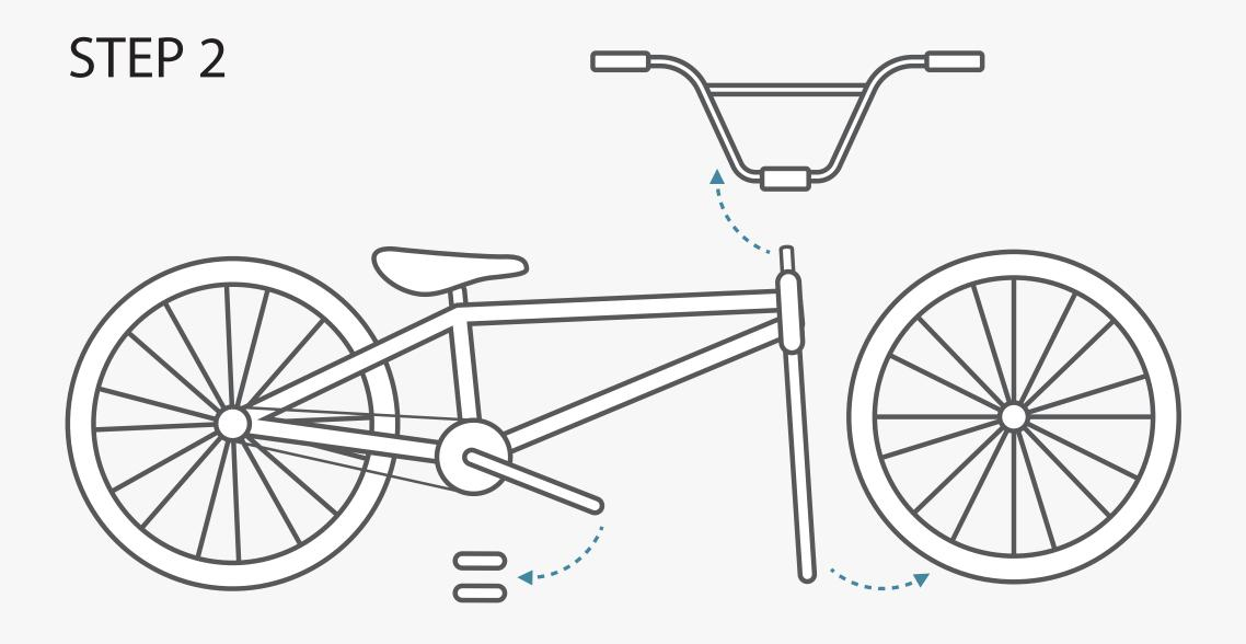
Carefully remove the pedals, the front rim and the handlebar.
