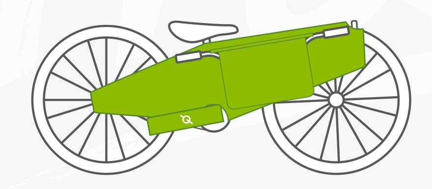
Place the handlebar on the Travel Pad (A) and then the BAG (B) as indicated by the image. You can adjust the briefcase (B) by pulling the strips to your liking.
