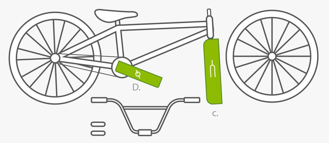
Place the fork protector (C) and the cranks (D) as the image indicates
