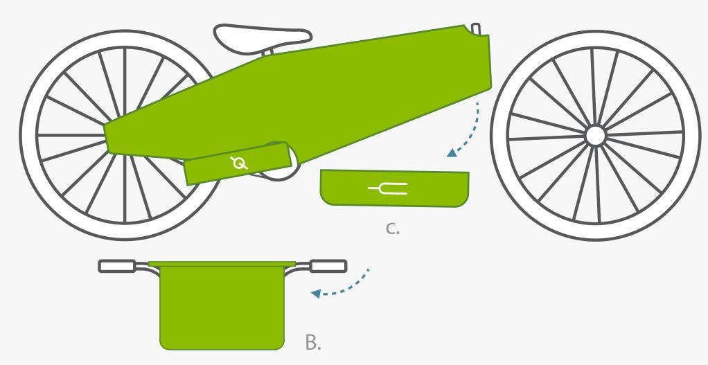
Remove the fork and place the pedals and tools inside the bag (B), as indicated by the image.
